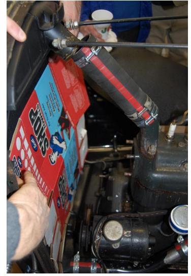
forward. Take care as you remove the pump not to damage the radiator fins, this is why the cardboard or other protectant is important.
