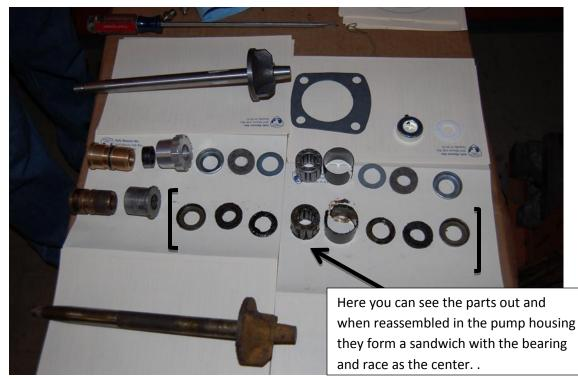
4. The rear bearing must be pressed out through the back of the housing. Add a little lubricant to aid in pressing out the bushing.
