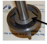
Impeller Bushing. 2 TYPEs Brass Square, 28-29, Steel Tear Drop, 30-31
